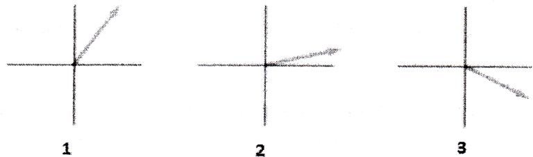
12- The corresponding figures (1,2 and 3) represents the instantaneous voltage across the elements of the RLC circuit respectively
