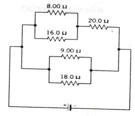
3) Using Kirchhoff's rules, (a) find the current in each resistor in the circuit. (b) Find the potential difference between points c and  $f(V_f - V_c)$ . Which point is at the higher potential?
