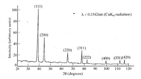
P6: Using Bragg's law, calculate the diffraction angles (20) for (111), (200) and (220) planes for Aluminum which is an fcc metal of lattice constant a = 4.04 Å. The wavelength of used X-ray  $\lambda = 1.542$  Å. (4 marks)
