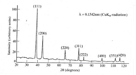
P6: Using Bragg's law, calculate the diffraction angles (20) for (111), (200) and (220) planes for Aluminum which is an fcc metal of lattice constant a = 4.04 Å. The wavelength of used X-ray  $\lambda = 1.542$  Å. (7 marks)
