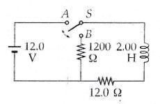
(b) Now the switch is thrown quickly from A to B. Compute the initial voltage across each resistor and across the inductor.
