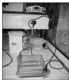
Gel tank (to place the gel mold and run electrophoresis)
