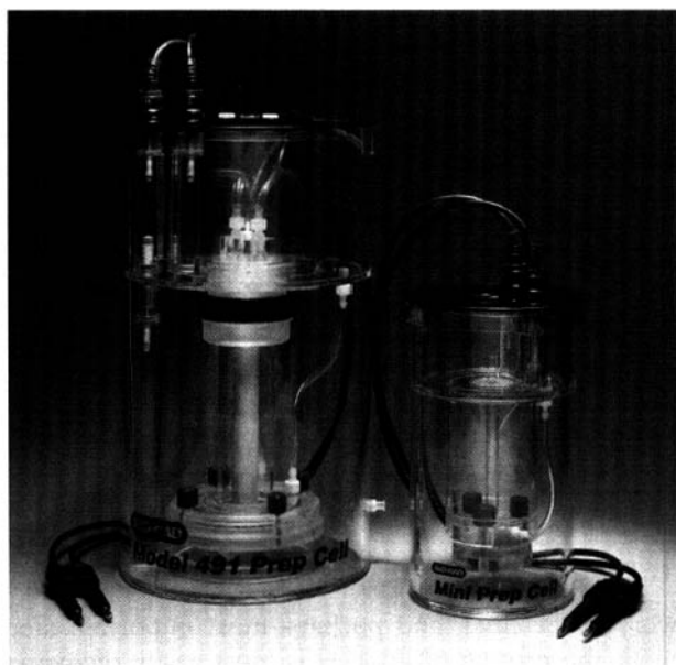
Figure 2. (a) Schematic depiction of the use of the Bio-Rad Model 491 Prep Cell for preparative electrophoresis. (b) The Model 491 Prep Cell.
