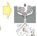
Force cells through a small hole using high pressure.
