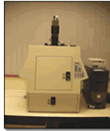
Gel documentation (capture and print the image of agarose gel)
