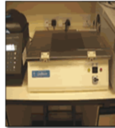
UV transilluminator (basic device for visualizing fluorescence-stained gels)
