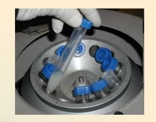
The interior of the centrifuge bowl should be inspected daily for staining or soiling at the level of rotors
