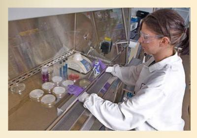
Apparatus and materials in the cabinet must be kept to minimum
