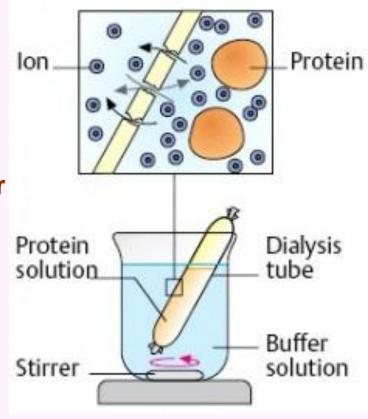
➤ After repeated exchanging of the external solution, the conditions inside the *dialysis tube* (salt concentration, pH, etc.) will be the same as in the surrounding solution.
