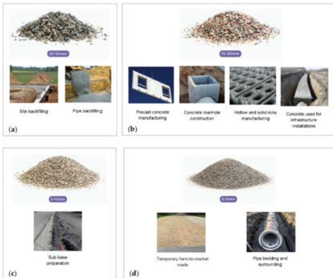
Figure 8. Pictorial vignettes of recycled aggregates and their potential uses. (a) 20–50 mm aggregates, (b) 10–20 mm aggregates, (c) 5–10 mm aggregates, and (d) 0–5 mm aggregates. (Source: SIRCI [16]).
